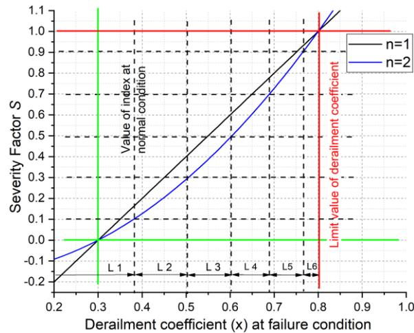
**Figure 54 - Example of severity factor  $s$  for derailment coefficient**
