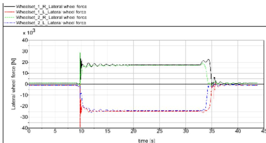
Figure 147 - Wheel lateral forces for passive IRW vehicle (without track irregularities)
