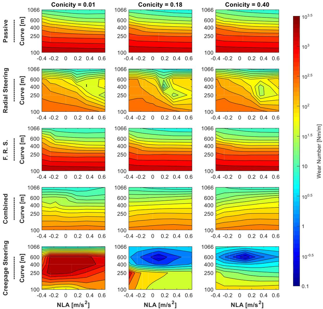
Figure 122 - Rear wheelset wear distribution - Feedback approach
