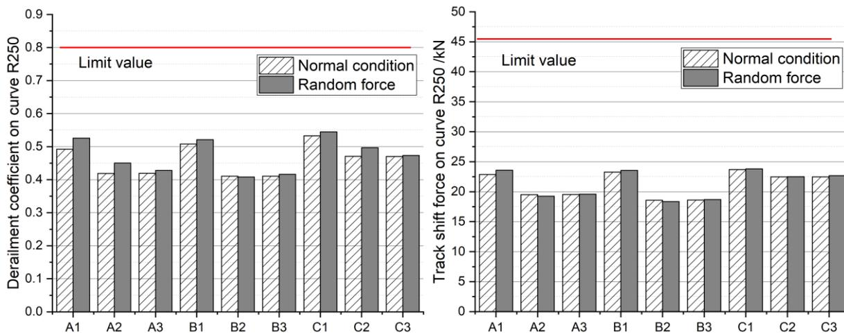
Figure 68 - (a) Derailment coefficient and (b) track shift force on curve R250 in normal condition and Random force
