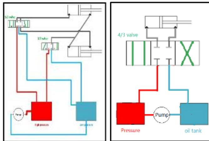
**Figure 56 - Interconnected and simple actuator models**
