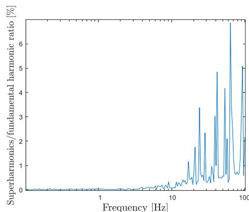
**Figure 97 - Ratio between the sum of the superharmonic amplitudes and the amplitude of the fundamental harmonic of the force vs the frequency of the command variable  $\xi$**
