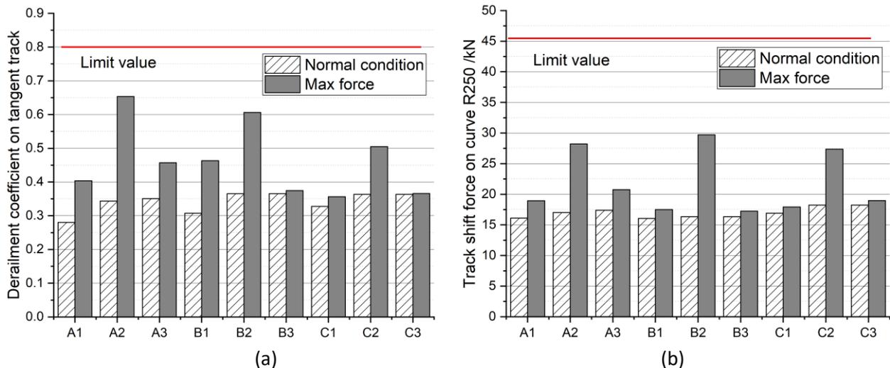
Figure 65 - (a) Derailment coefficient and (b) track shift force on tangent track in normal condition and Maximum force
