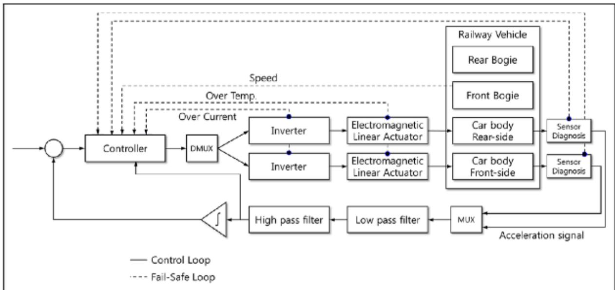
Figure 19 - Fail-safe control scheme for active lateral suspension system [68]
