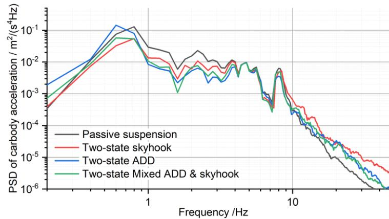
**Figure 83 - PSD analysis on the effects of two-state control strategies**
