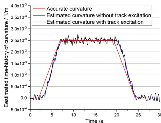
Figure 43 - Comparison between the accurate curvature and estimated curvature
