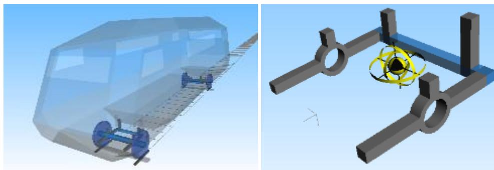
Figure 106 - MBS vehicle model (left) and frame model (right)
