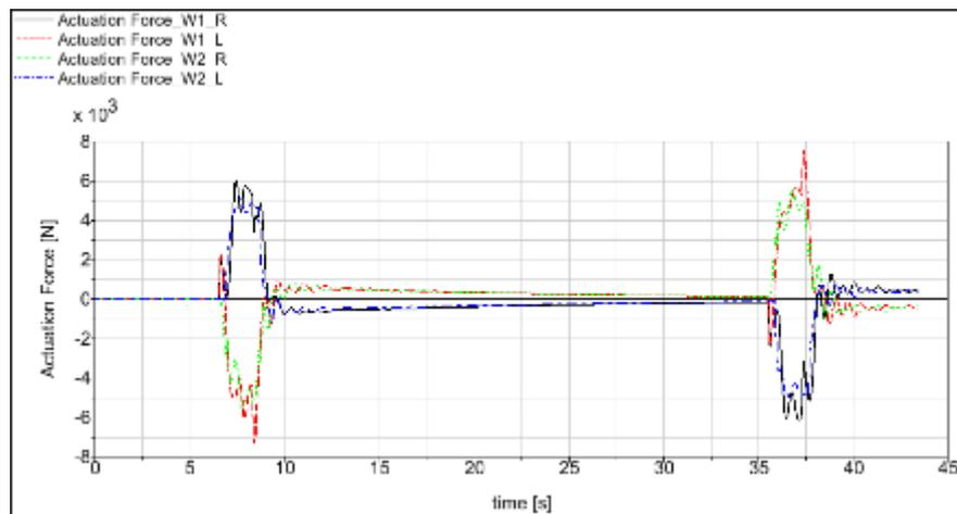
Figure 136 - Actuator Forces for yaw relaxation control (without track irregularities)
