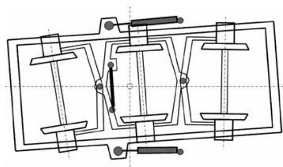
**Figure 30 - Actuated yaw force steered bogie (AY-FS)**
