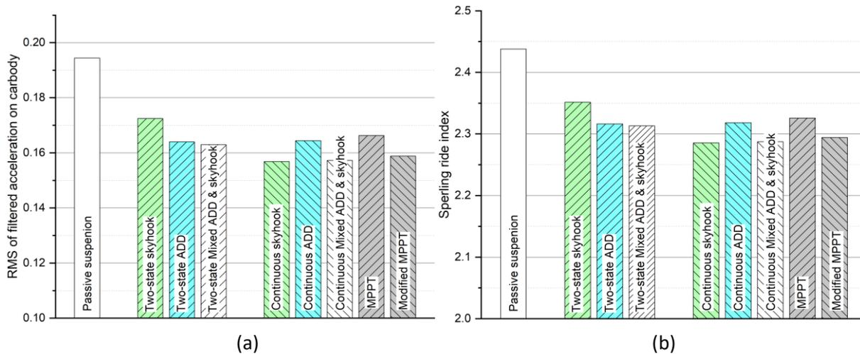
Figure 85 - Simulation results of (a)RMS value and (b)Sperling ride index with different control strategies
