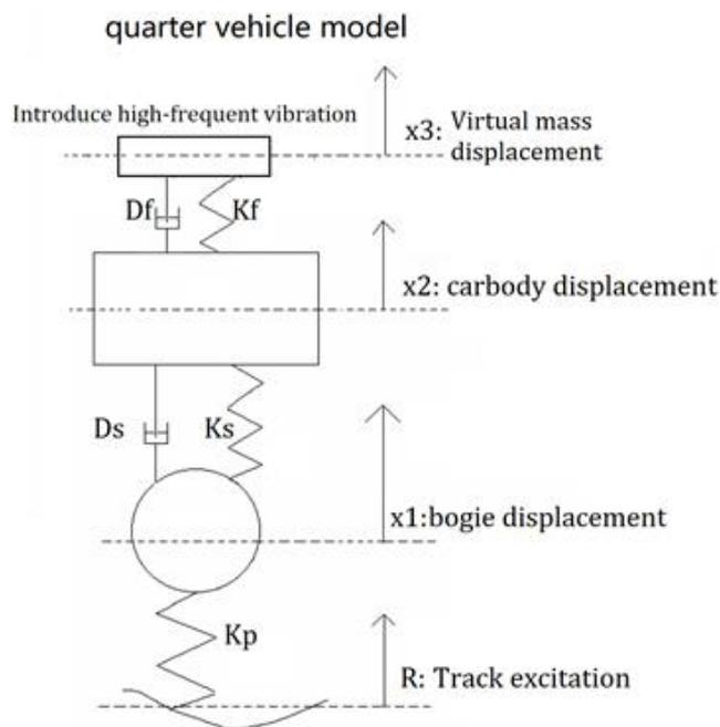
Figure 72 – Modified one-quarter vehicle model
