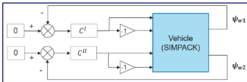
Figure 117 - Radial steering control scheme
