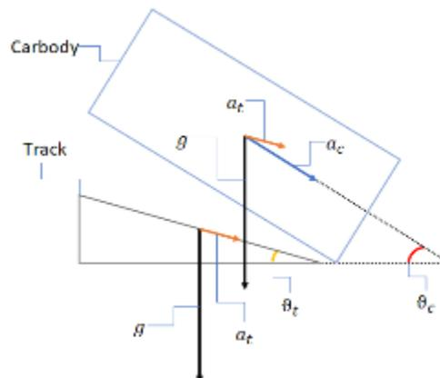
**Figure 110 - Sway model calculation**
