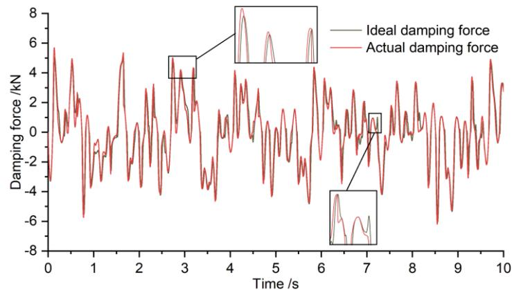
Figure 80 - Ideal damping force and actual damping force with Two-state Skyhook in one-quarter vehicle model
