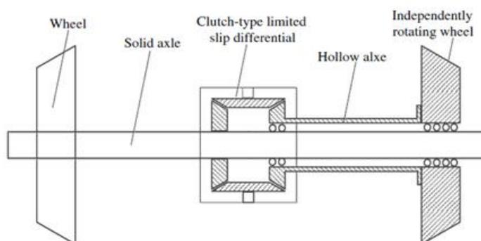
Figure 36 - Differential coupling wheelset [106]
