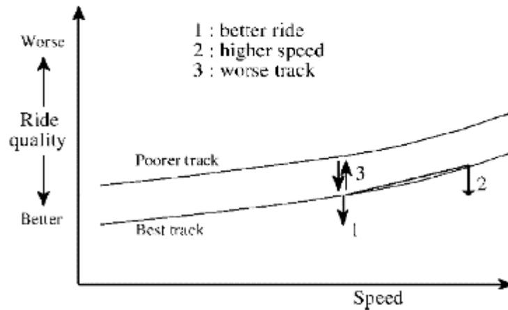
Figure 8 - The applicable backgrounds for active secondary suspension [4]
