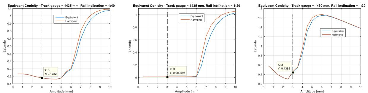
**Figure 113 - Conicity profiles: case a (left), case b (center) and case c (right)**
