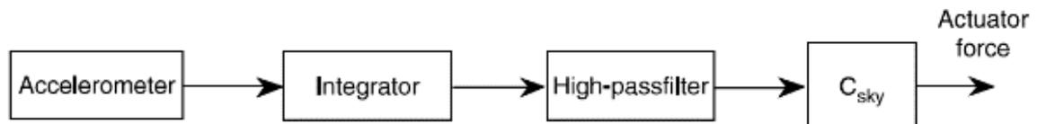
Figure 14 - The workflow for sky-hook damper [28]
