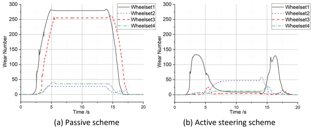
Figure 47 - Wheelset wear number with no track irregularity
