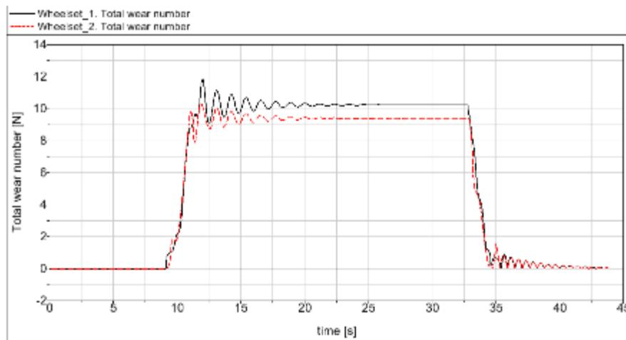
Figure 155 - Wheelset total wears for dual-loop-control motorized IRW (without track irregularities)
