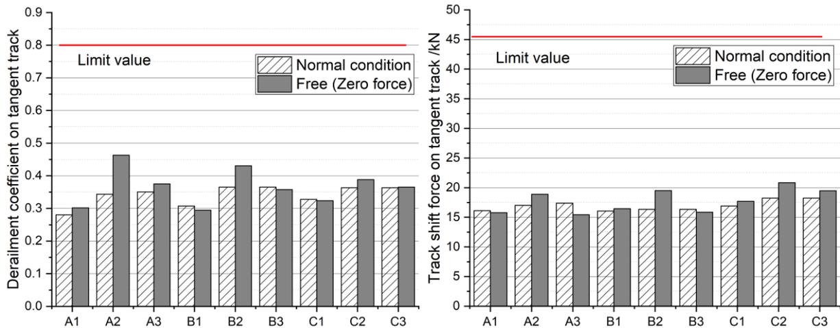
Figure 69 - (a) Derailment coefficient and (b) track shift force on tangent track in normal condition and Free
