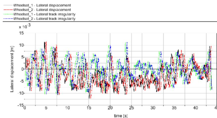
**Figure 158 - Wheelset lateral displacements for dual-loop-control non-motorized IRW and lateral track irregularities**
