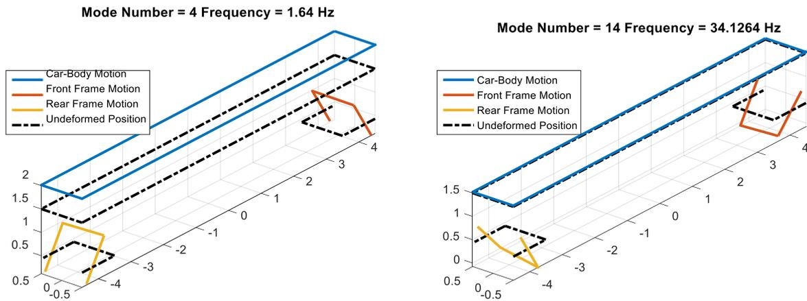
**Figure 166 - Modes shapes representation: 4th mode (left) and 14th mode (right)**
