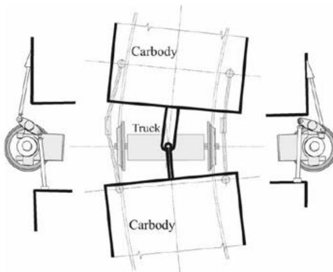
Figure 35 - Talgo's Steering Mechanism [105]
