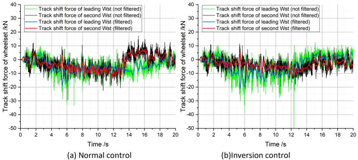
Figure 63 - Time history of track shift force for scheme B3 in (a) normal control and (b) Inversion control
