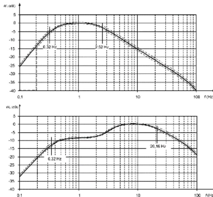
Figure 12 – Lateral (top) and vertical (bottom) weighting curves, EN 12299 [24]
