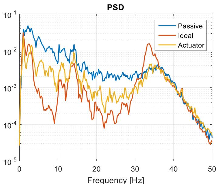
**Figure 168 - Modelled vs Ideal actuator vertical modal control acceleration PSD**
