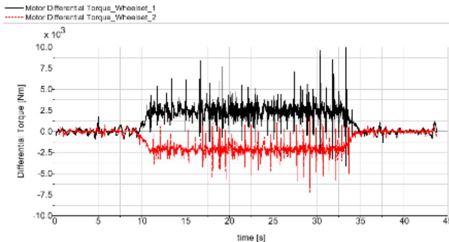
Figure 156 - Differential motor torques for dual-loop-control motorized IRW (with track irregularities)
