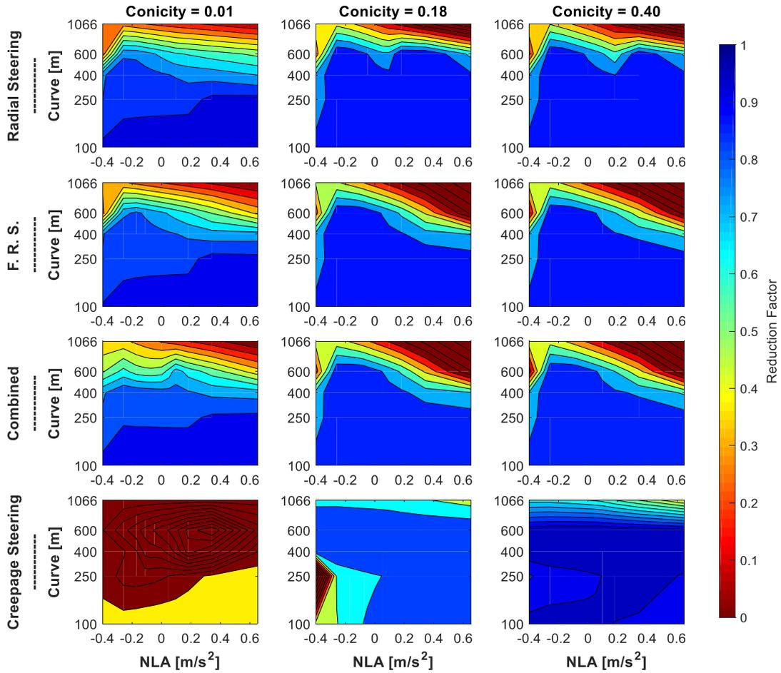
Figure 123 - Front wheelset wear reduction distribution - Feedback approach
