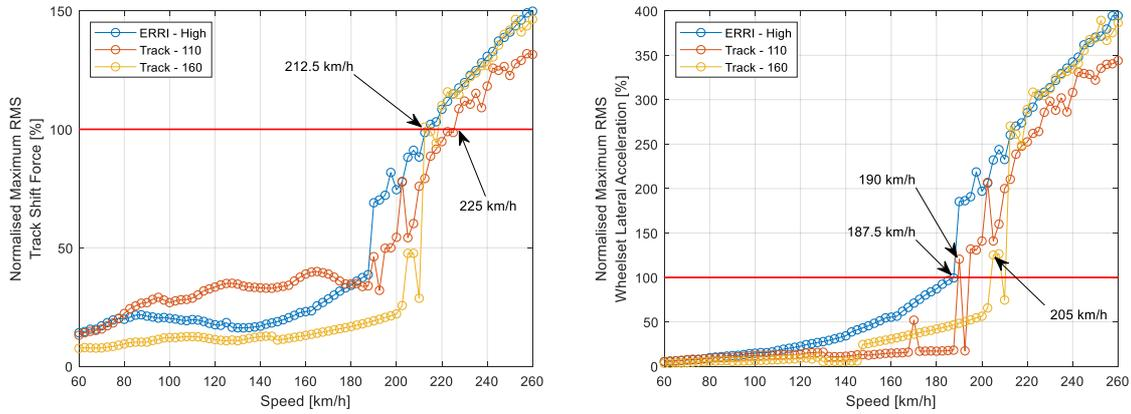
Figure 114 - Stability assessment, case a): track shift force (left), wheelset acceleration (right)
