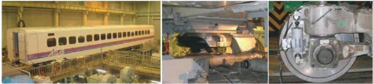
Figure 22 - Test Plant (left), Air spring (centre) and axle damper (right) [31]
