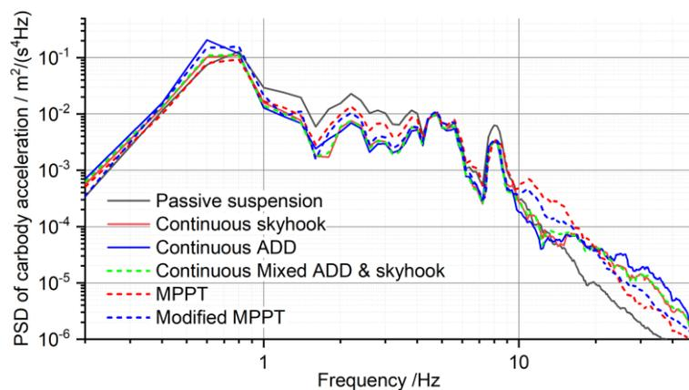
Figure 87 - PSD analysis on the effects of continuous control strategies
