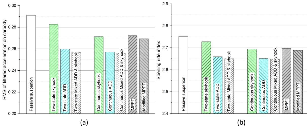
Figure 92 - Simulation results of (a)RMS value and (b)Sperling ride index with different control strategies
