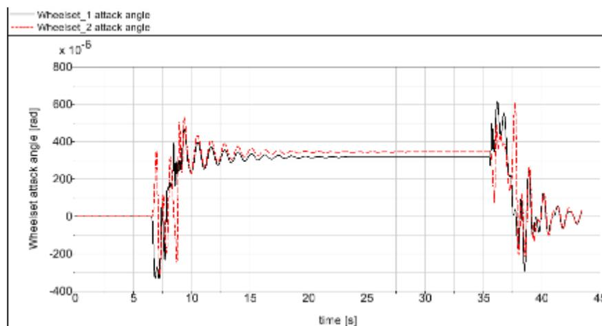
Figure 135 - Wheelset attack angles for yaw relaxation control (without track irregularities)
