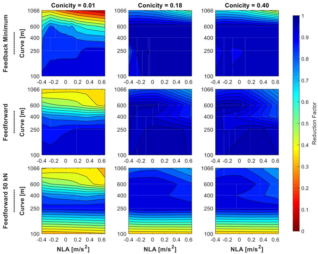
Figure 128 - Front wheelset wear reduction distribution - Feedforward approach
