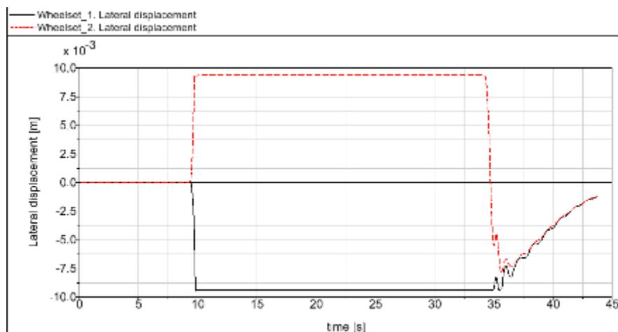
Figure 146 - Wheelset lateral displacements for passive IRW vehicle (without track irregularities)
