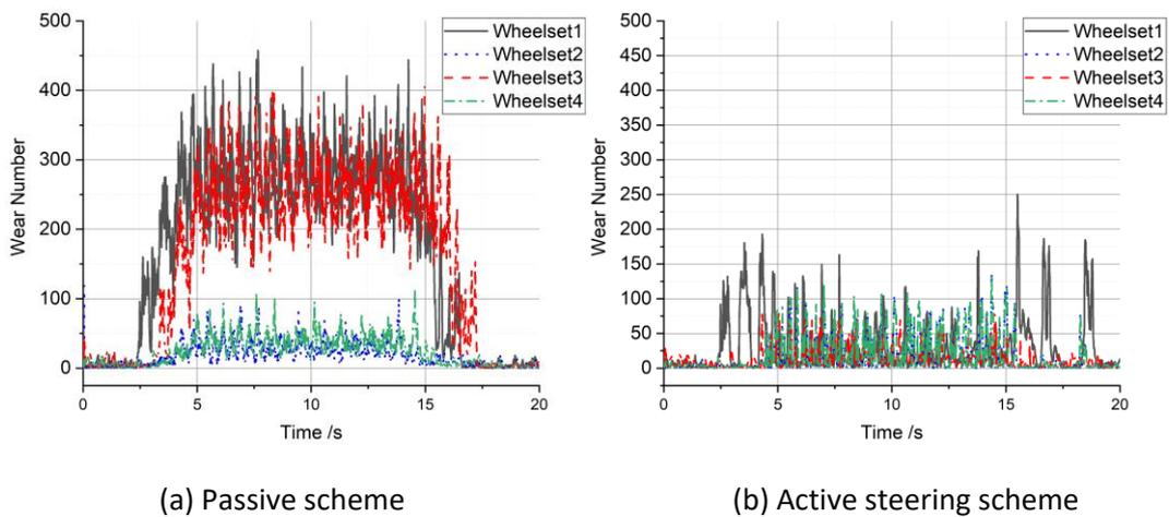
**Figure 50 - Wheelset wear number with track irregularity**
