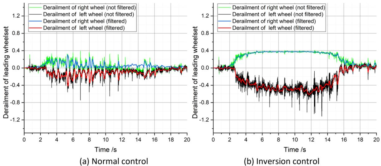
**Figure 59 - Time history of derailment coefficient (Y/Q) for scheme B2 in (a) normal control and (b) Inversion control**
