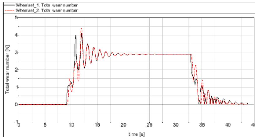
Figure 161 - Wheelset total wears for dual-loop-control non-motorized IRW (without track irregularities)
