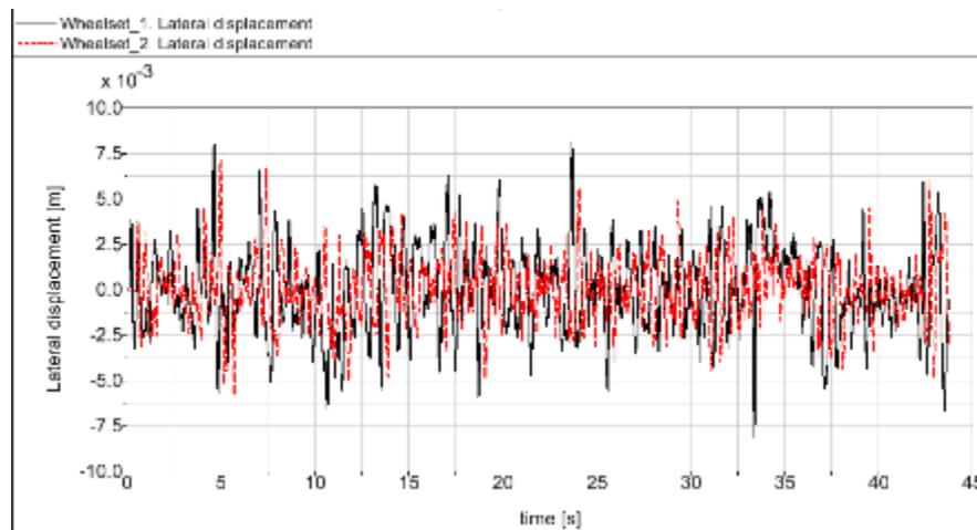
**Figure 152 - Wheelset lateral displacement for tri-loop-control motorized IRW (with track irregularities)**
