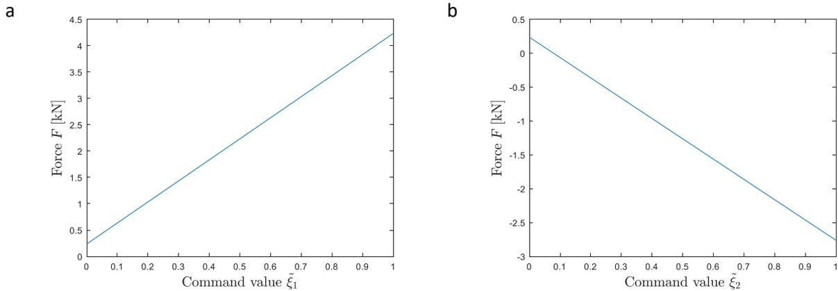
**Figure 95 - Static force as a function of the command value**
