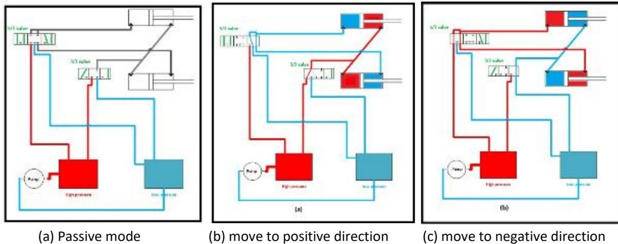
Figure 39 - Inter-connected hydraulic actuator model and its working modes
