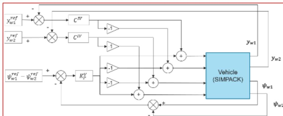
Figure 120 - Creepage steering control scheme
