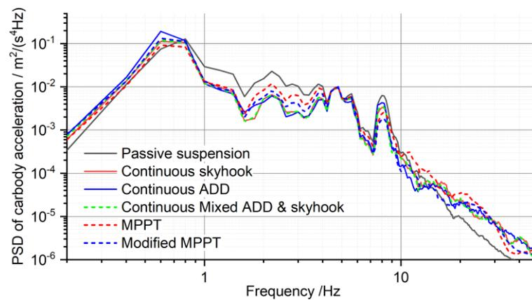
**Figure 84 - PSD analysis on the effects of continuous control strategies**
