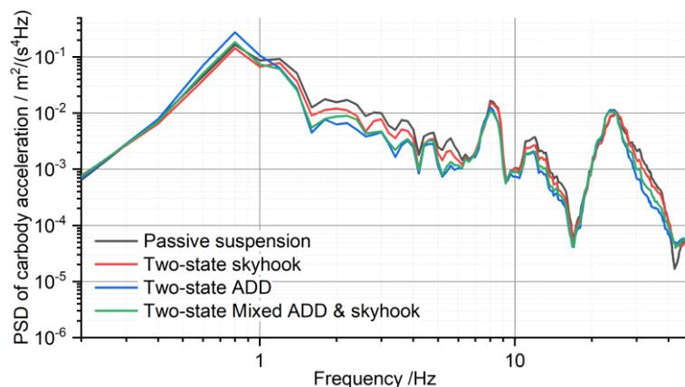
Figure 89 - PSD analysis on the effects of two-state control strategies
