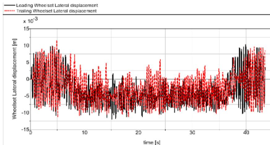
**Figure 130 - Wheelset lateral displacements for passive solid-axle vehicle with low yaw stiffness (with track irregularities)**
