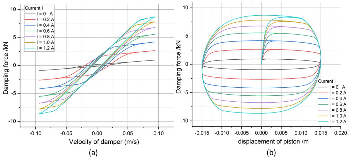
**Figure 75 - The (a) force-velocity feature and (b) force-displacement feature of the MR damper**
