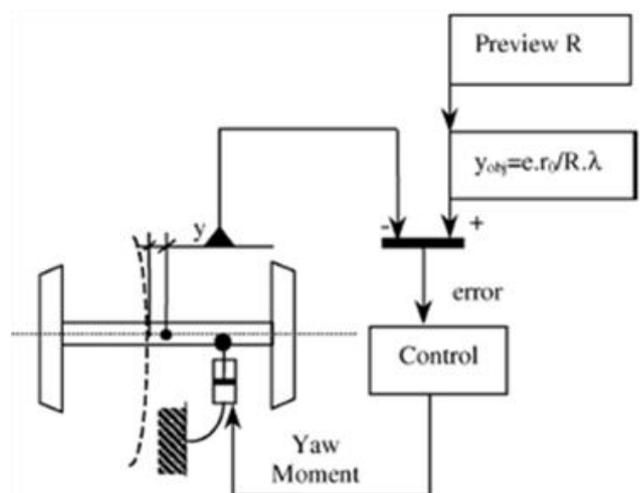
Figure 31 - Control strategy based on lateral position of wheelset as control target
