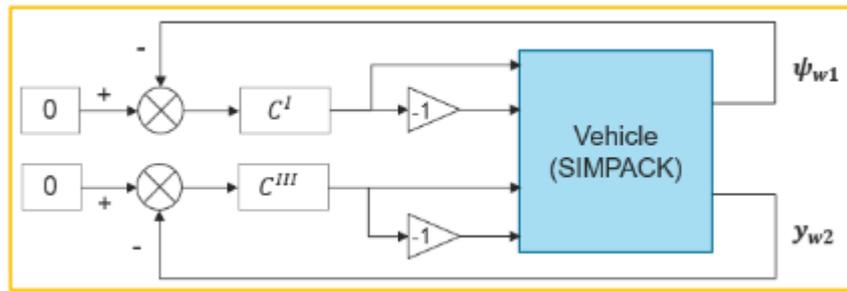
Figure 119 - Combined steering control scheme
