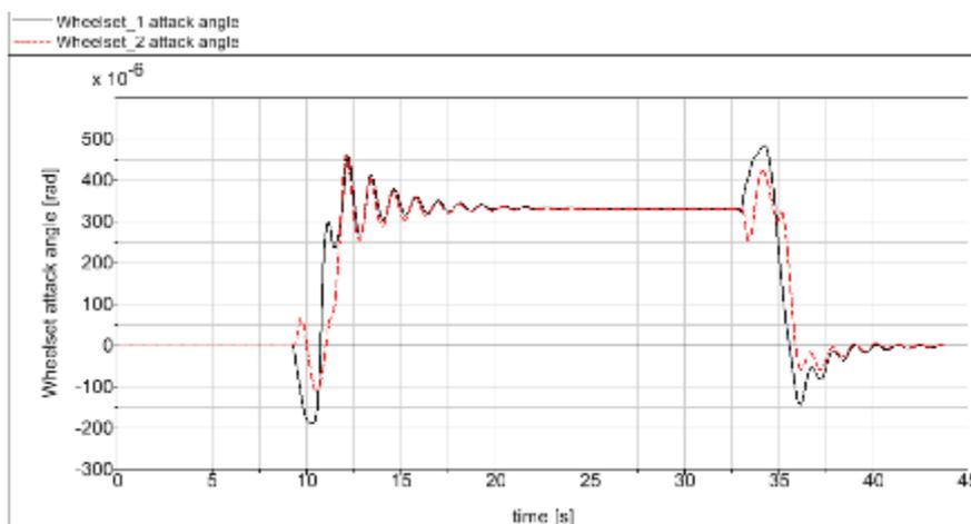
Figure 160 - Wheelset attack angles for dual-loop-control non-motorized IRW (without track irregularities)
