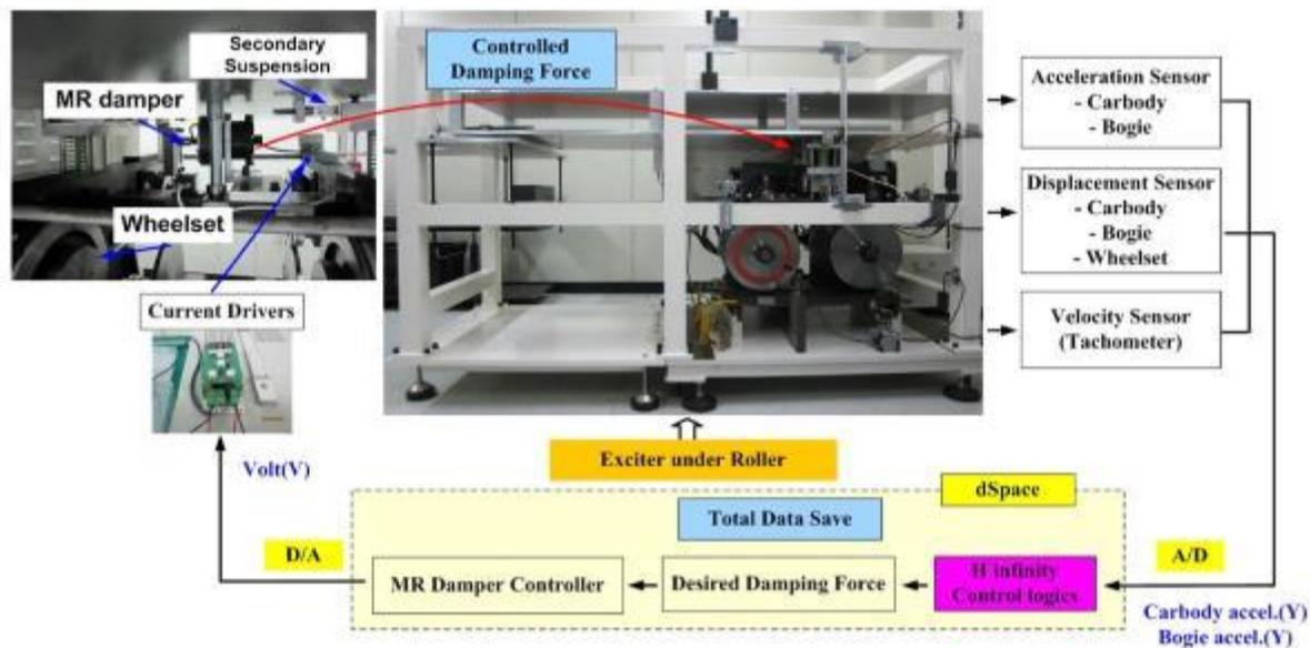
Figure 24 - Measurements and control loop for 1:5 scale roller rig test [77]
