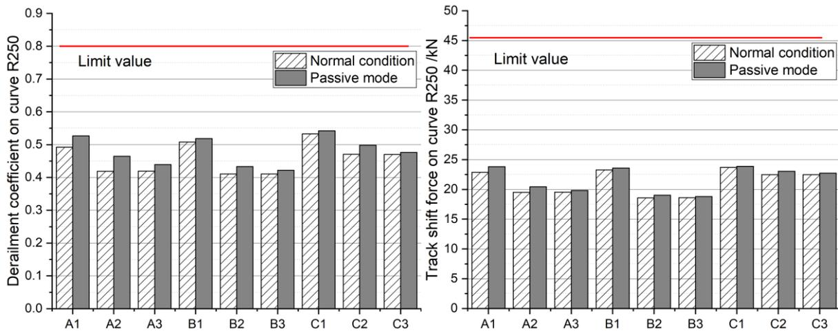
Figure 71 - (a) Derailment and (b) track shift force on curve R250 in normal condition and Passive mode
