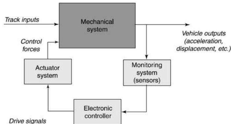
Figure 1 - Workflow of active suspension [5]
