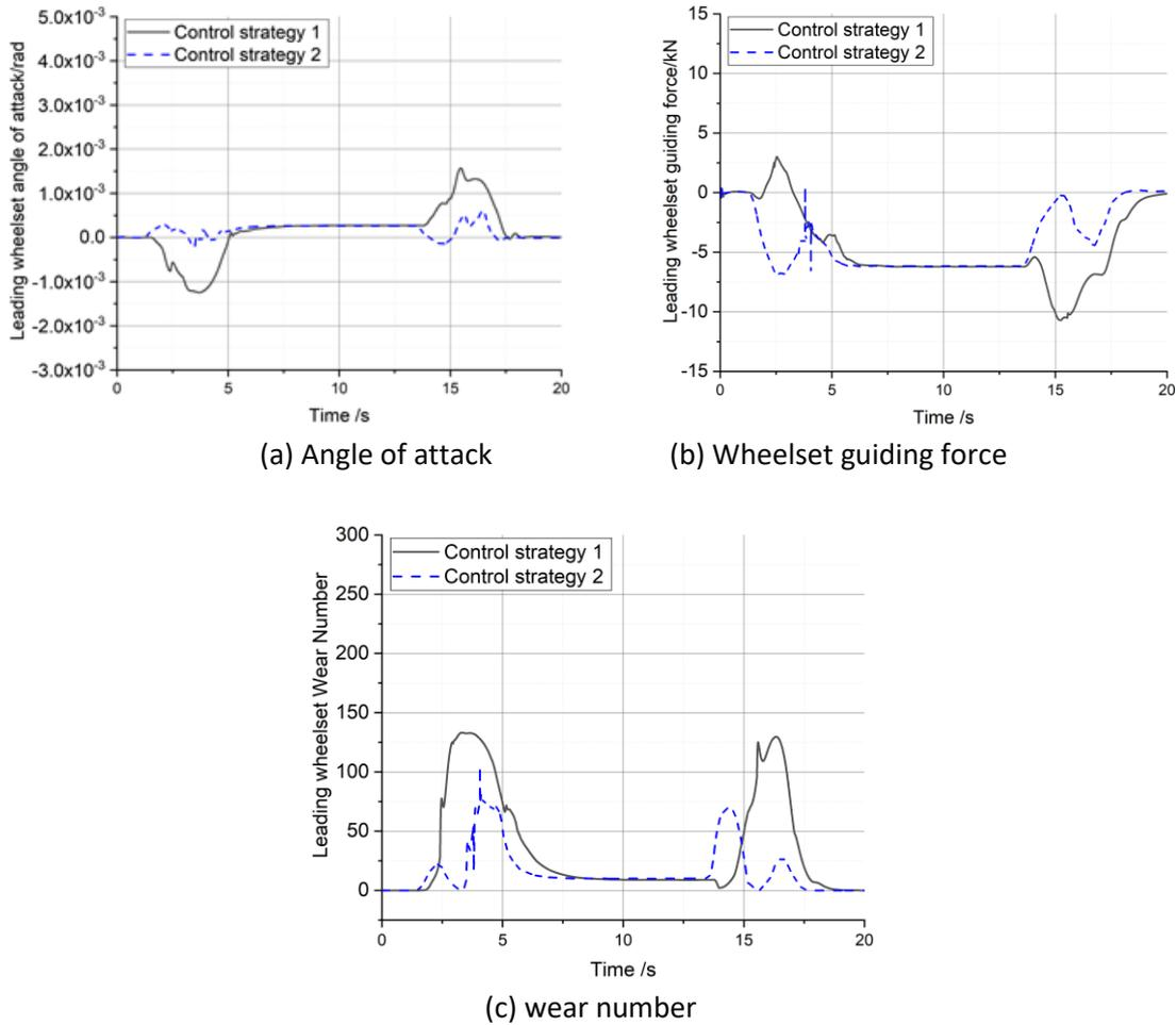
**Figure 52 - Performance of leading wheelset with two control strategies (no track irregularity)**
