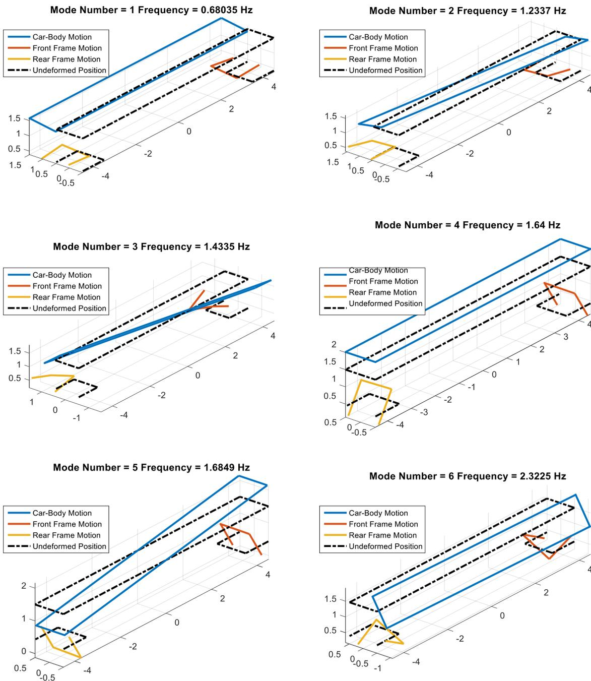
Figure 175 - Two-axle vehicle first six modes
