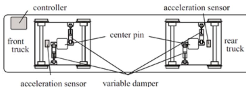
Figure 25 - Set-up of the semi-active system used for test train WIN350 [69]
