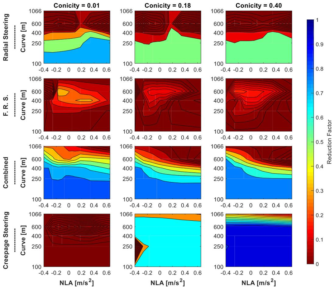
Figure 124 - Rear wheelset wear reduction distribution - Feedback approach
