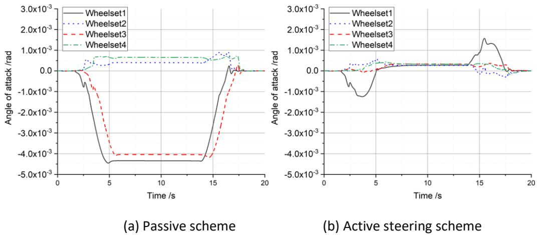
Figure 45 - Wheelset angle of attack with no track irregularity
