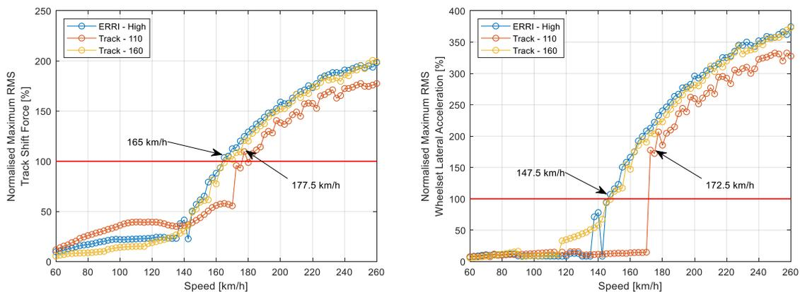
Figure 116 - Stability assessment, case c): track shift force (left), wheelset acceleration (right)
