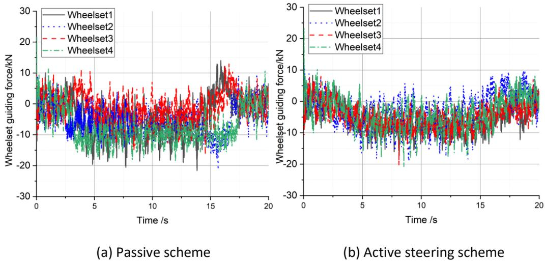
**Figure 49 - Wheelset guiding force with track irregularity**
