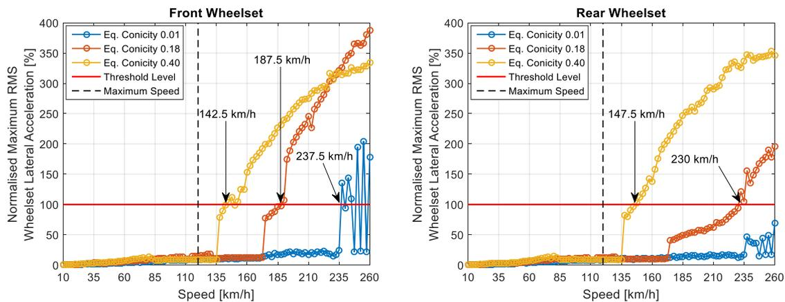
Figure 141 - HALL stability assessment - Acceleration front (left) and rear (right) wheelset
