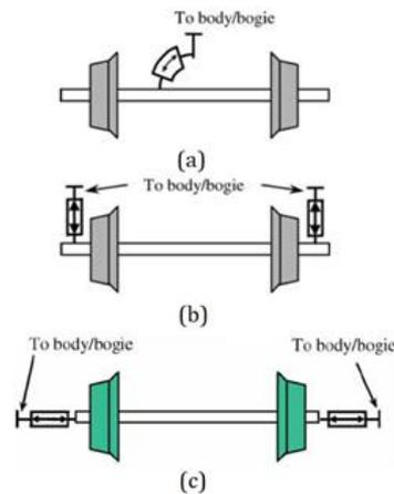
Figure 27 - Mechanical schemes for solid-axle wheelsets
