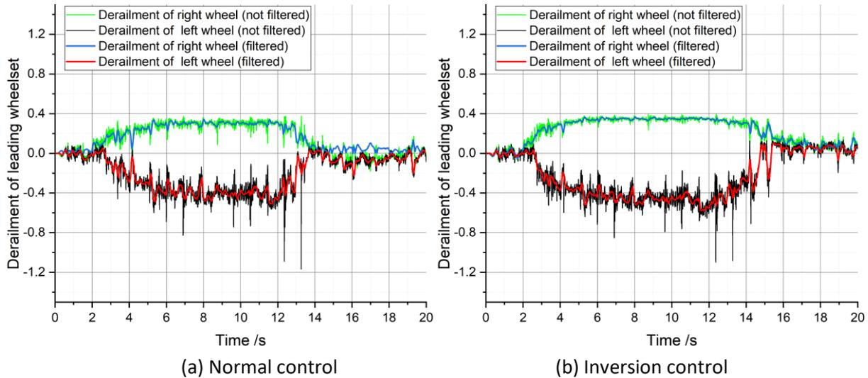
**Figure 58 - Time history of derailment coefficient (Y/Q) for scheme B1 in (a) normal control and (b) Inversion control**
