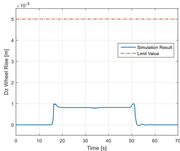
Figure 111 - Twisted track assessment EN14363 [128] - method 1
