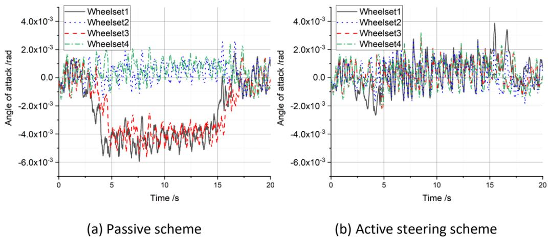
Figure 48 - Wheelset angle of attack with track irregularity
