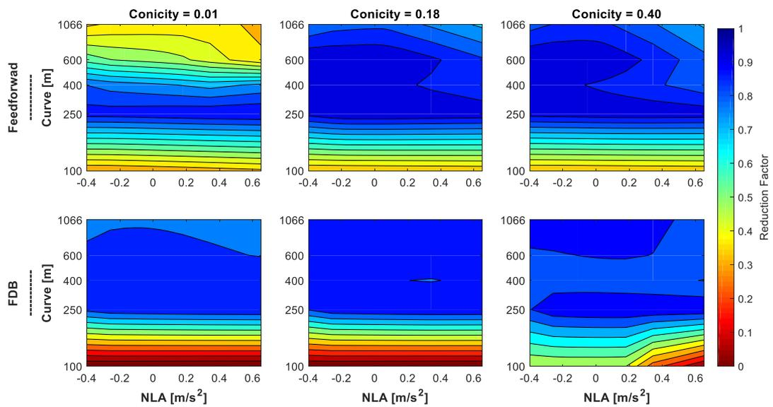
Figure 144 - Front wheelset wear reduction distribution - HALL bush
