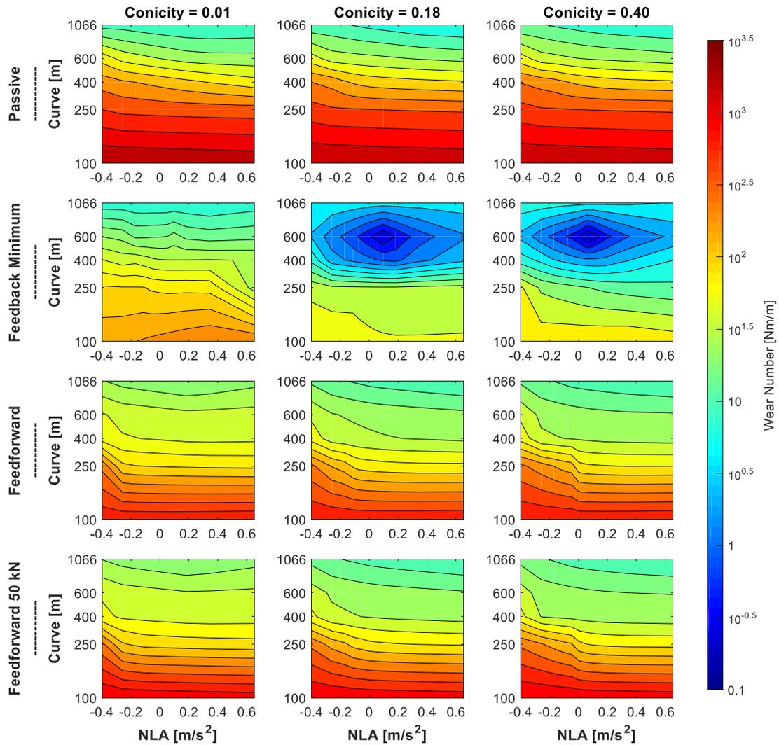
Figure 127 - Rear wheelset wear distribution - Feedforward approach
