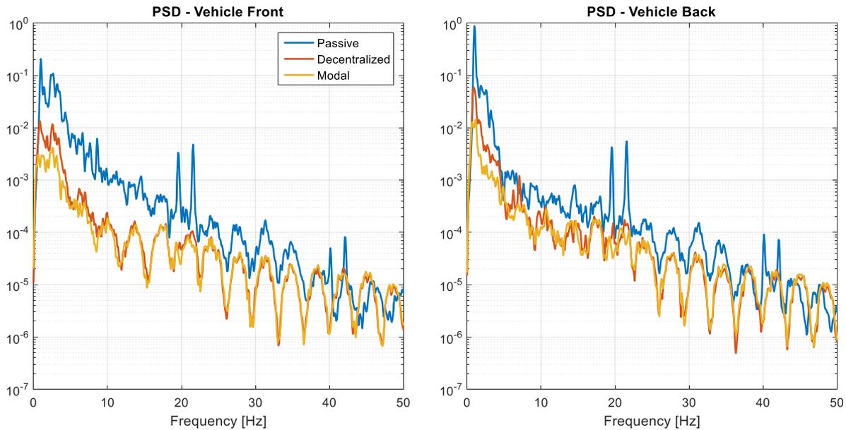
**Figure 173 - Lateral comfort control comparison**
