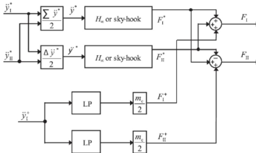
Figure 18 - Modal control considering lateral and yaw motion with conjunction of HOD [53]
