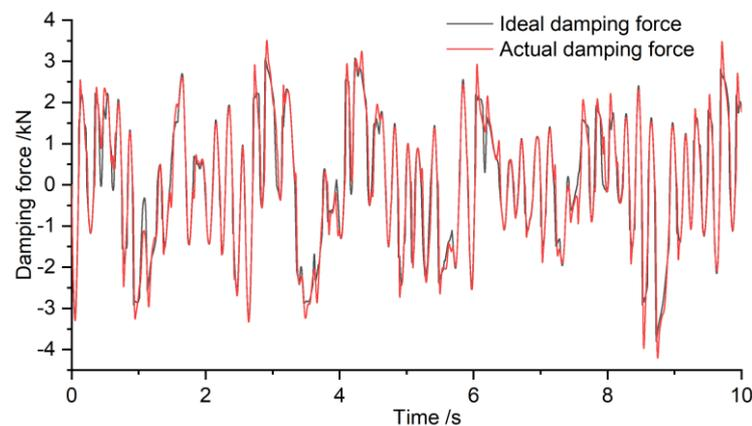
Figure 81 - Ideal damping force and actual damping force for Continuous Skyhook in one-quarter vehicle model
