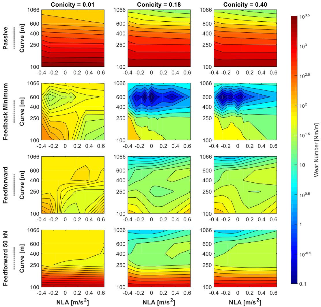
Figure 126 - Front wheelset wear distribution - Feedforward approach
