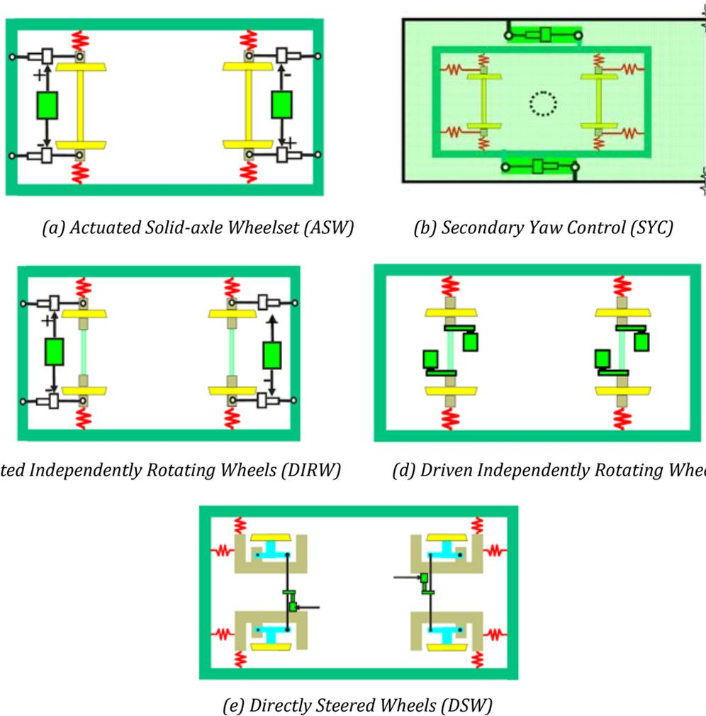
Figure 26 - Five configurations for active primary suspension
