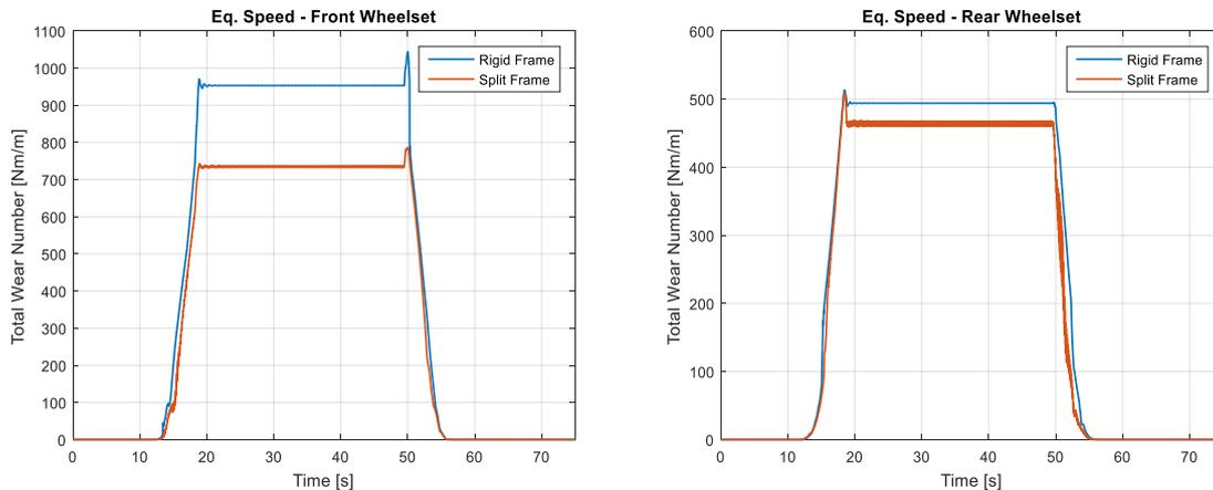
**Figure 109 - Comparison of wear numbers at curve negotiation, rigid against split frame: front wheelset (left) and rear wheelset (right)**
