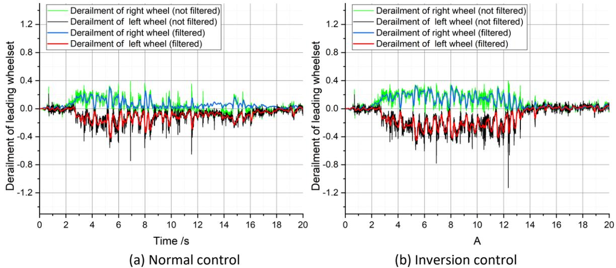
**Figure 60 - Time history of derailment coefficient ( $Y/Q$ ) for scheme B3 in (a) normal control and (b) inversion control**
