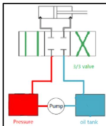
Figure 40 - The principle of simple hydraulic actuator
