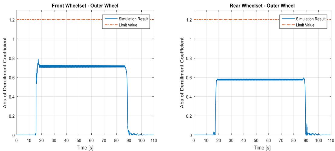
Figure 112 - Twisted track assessment EN14363 [128] - method 2
