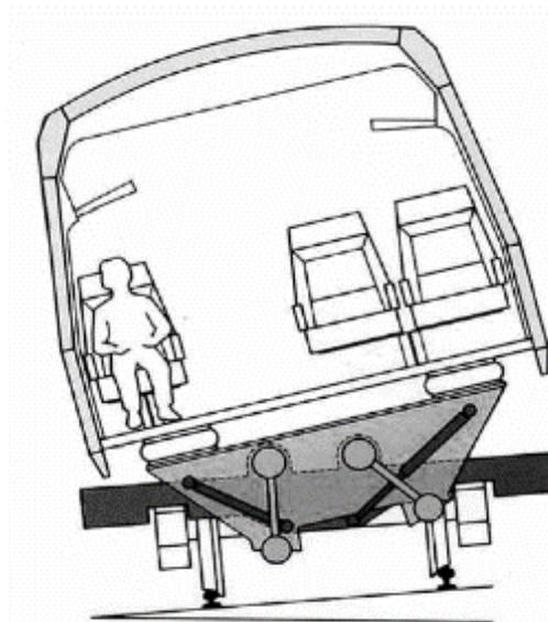
Figure 6 - Active Tilt Mechanism [6]
