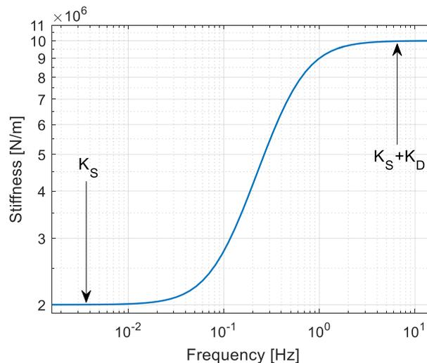
Figure 139 - Hydraulic bush frequency behaviour
