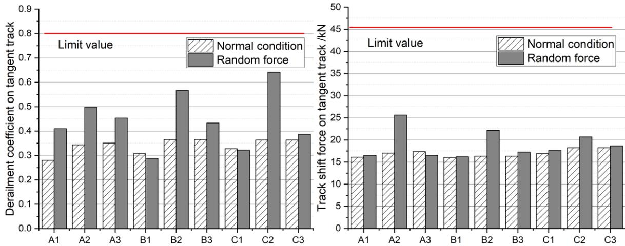
Figure 67 - (a) Derailment coefficient and (b) track shift force on tangent track in normal condition and Random force
