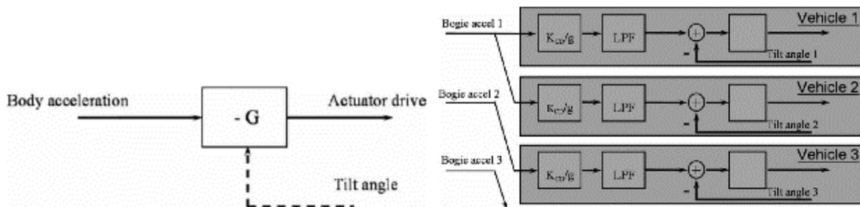
Figure 7 - Tilting Controls: nulling control (left), precedence control (right) [6]
