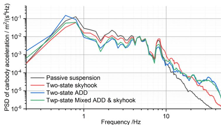
Figure 86 - PSD analysis on the effects of two-state control strategies
