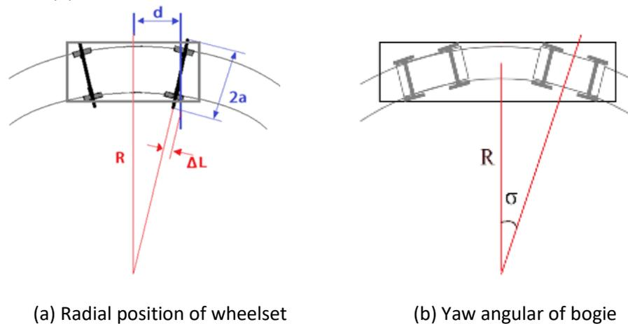
Figure 42 – Radial position of wheelset and yaw angle of bogie
