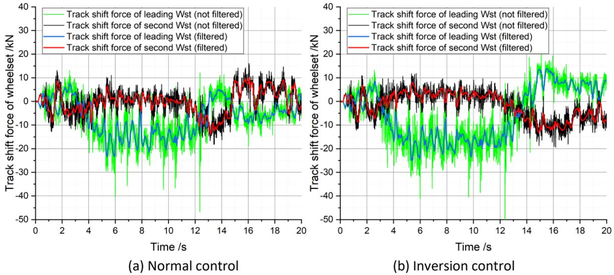
Figure 61 - Time history of track shift force for scheme B1 in (a) normal control and (b) Inversion control
