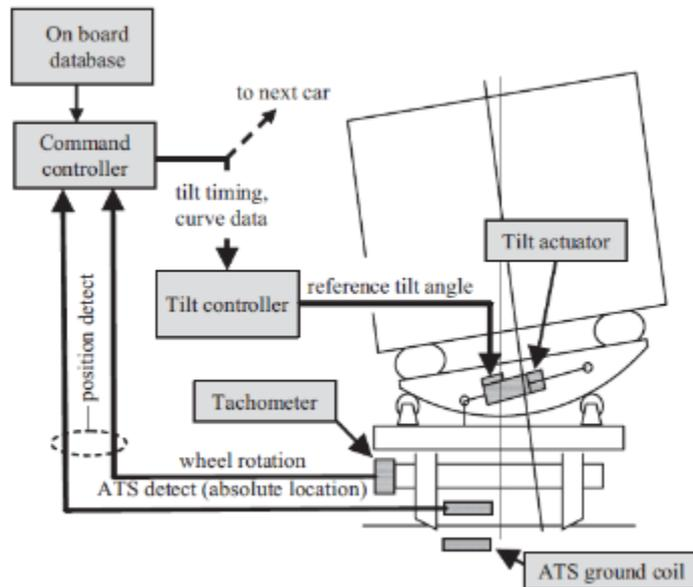
Figure 5 - Controlled Natural Tilting [6]
