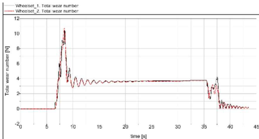
Figure 137 - Wheelset wear indexes for yaw relaxation control (without track irregularities)
