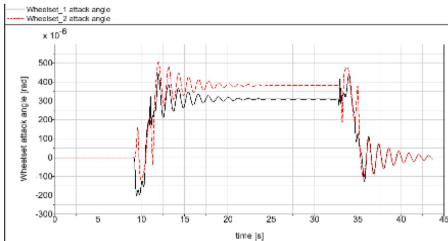
Figure 154 - Wheelset attack angles for dual-loop-control motorized IRW (without track irregularities)
