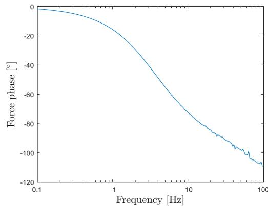
**Figure 98 - Phase of the force fundamental harmonic with respect the command variable  $\xi$  , vs the frequency of the command variable**
