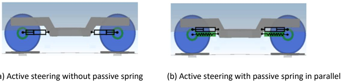
Figure 41 - Arrangement of two active steering schemes
