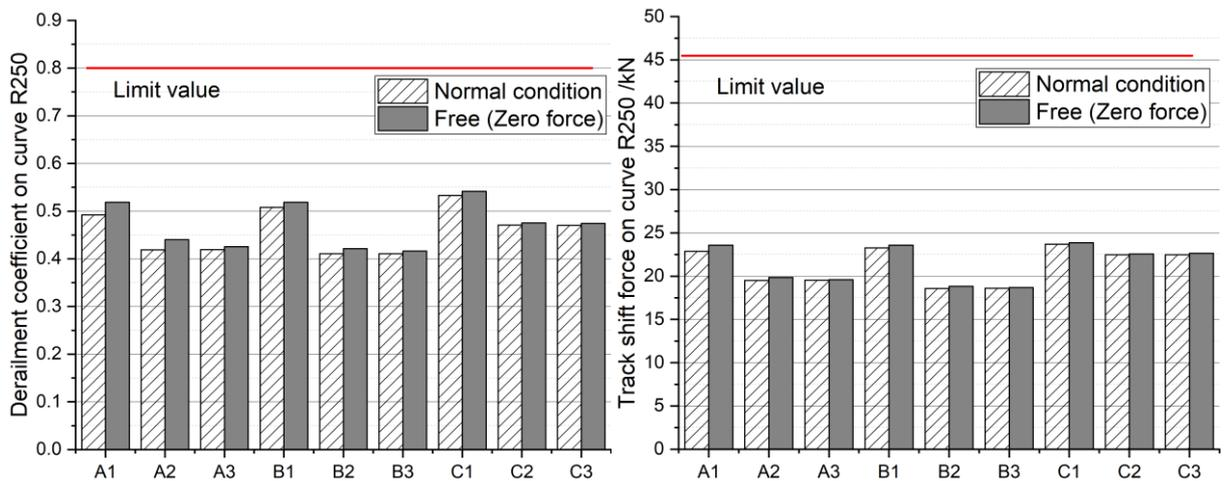
Figure 70 - (a) Derailment coefficient and (b) track shift force on curve R250 in normal condition and Free
