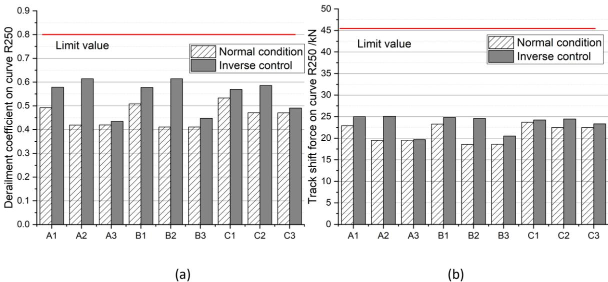
Figure 64 - (a) Derailment coefficient and (b) track shift force on Curve R250 in normal condition and Inverse control
