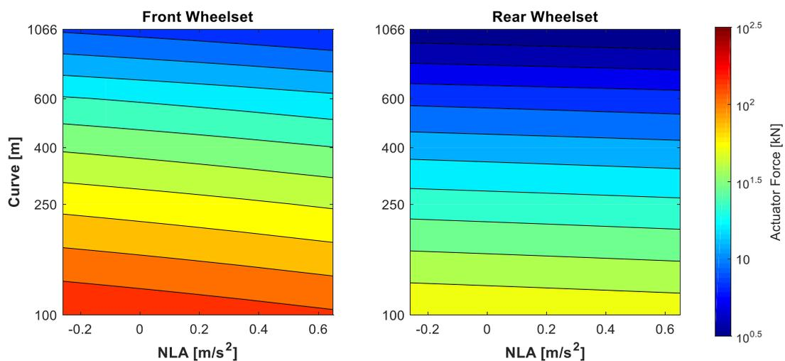
Figure 125 - Feedforward force distribution
