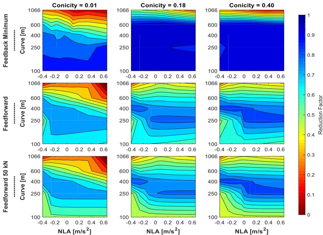
**Figure 129 - Rear wheelset wear reduction distribution - Feedforward approach**
