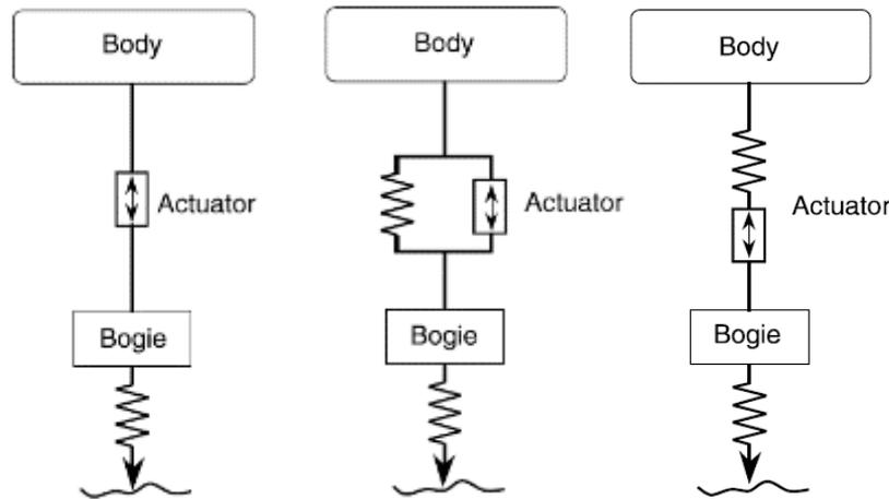
**Figure 10 - Mechanical configurations of active secondary suspension**
