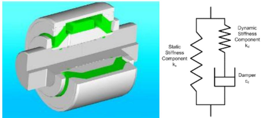
Figure 138 - Hydraulic bush (HALL): view (left) and model (right) [130]
