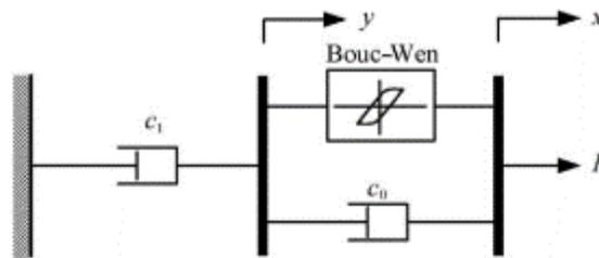
Figure 74 - Schematic of the modified Bouc-Wen model for MR damper [62]
