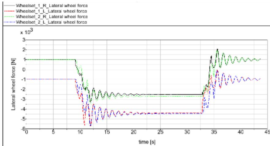
Figure 153 - Wheel/rail lateral forces for dual-loop-control motorized IRW (without track irregularities)
