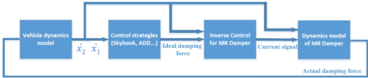
Figure 76 - The schematic workflow of the simulation considering the damper model
