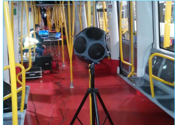
Fig. 10: Acoustic source inside the vehicle used to measure transmission through the carbody
