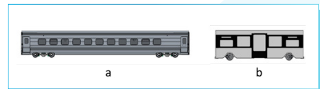
Fig. 6: The two concept vehicles a) bogie b) two axle
