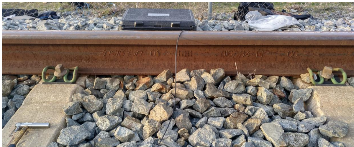
Figure 54: Rail fastening system in the test track.
