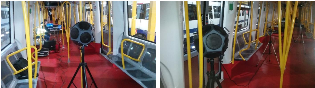
Figure 79: Reverberation time measurement. Different source and microphone locations.
