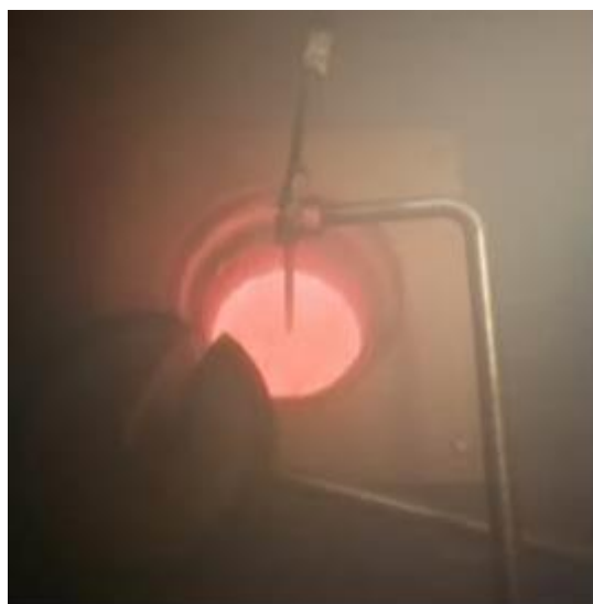
Figure 73: Induction furnace of RINA CSM's VIGA
