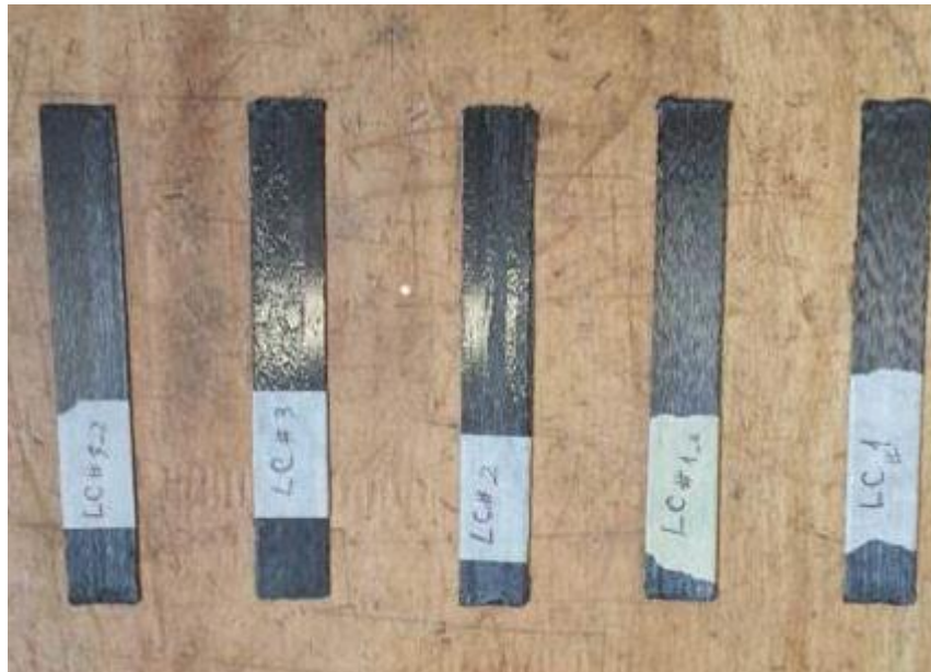
Figure 108: Samples printed on the TAZ with the Markforged filament and the new printing head
