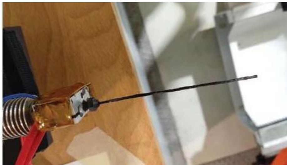
Figure 121: Manual consolidation of commingled yarn
