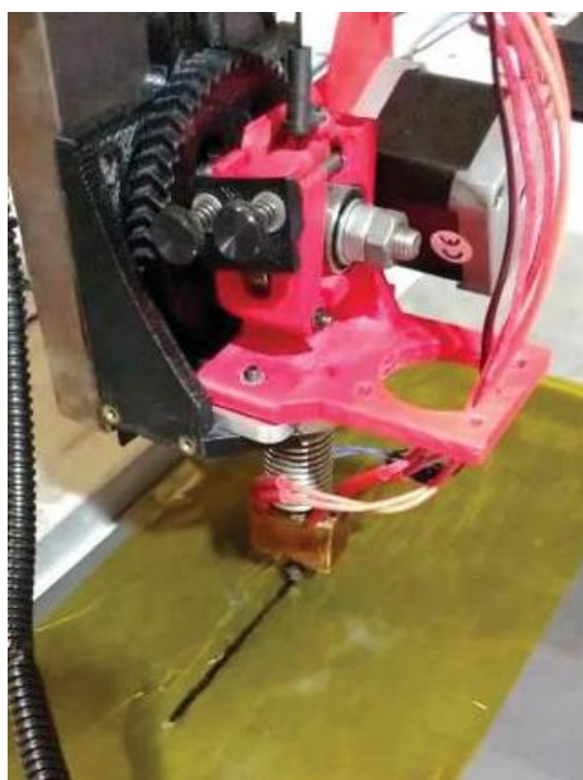
Figure 127: PA12 12k AS4A filament printing test
