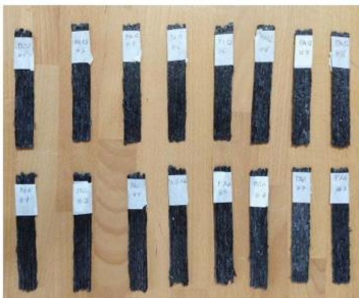
Figure 130: Samples of PA6 12k AS4A and PA12 12k AS4A
