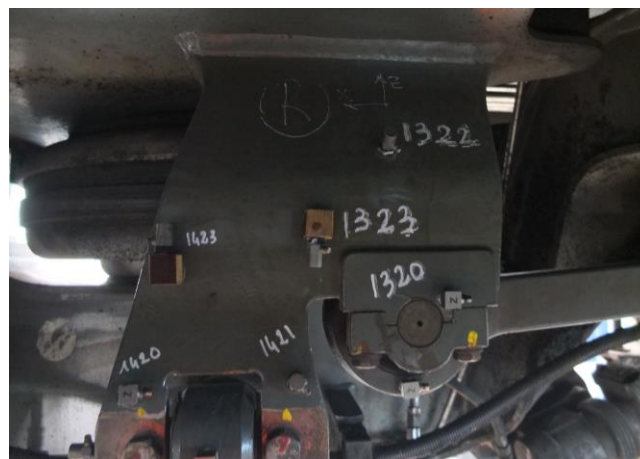
Figure 1: Carbody connection at the right side with accelerometers for TPA accelerance matrix
