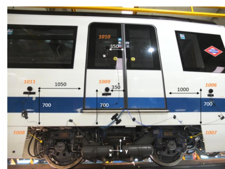
Figure 35: Microphone locations on the side of the train.
